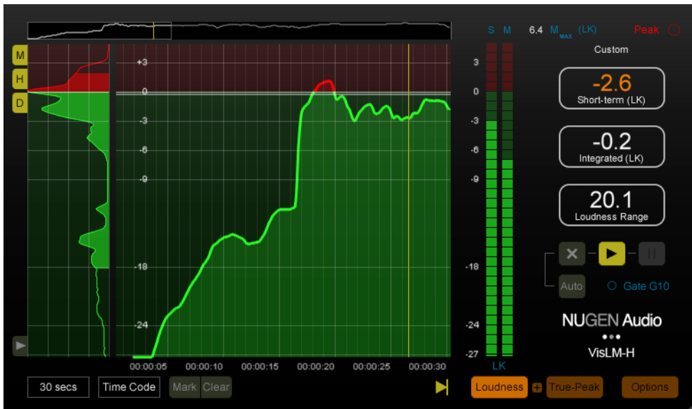
Fig 2. VisLM-H showing a 'green zone' Short-term Loudness range, with a no-go zone highlighted in red.
